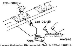
Limited Reflection Photoelectric Switch E3S–LS10XE4 Sensor Controller S3D8
